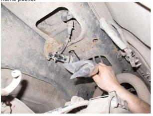
FIG 5, Ride Height Sensor secured Solenoid Tucked
