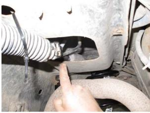
FIG 6, Pin connector for control module on 1991-1997 all models and 2000-2010 Crown Victoria & Grand Marquis
