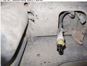
FIG 3, Solenoids and Ride Height Sensor
